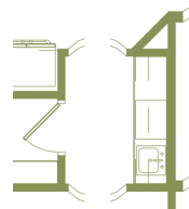
16 WET BAR W/ SINK AND REFRIGERATOR
